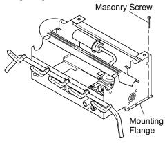
Figure 12 - Attaching Base Assembly to Fireplace Floor
